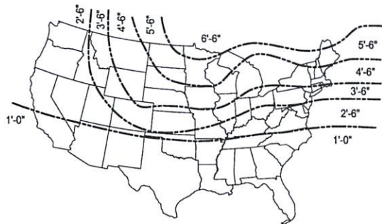
FOOTING DEPTH BELOW GRADE DIMENSION 'D'
